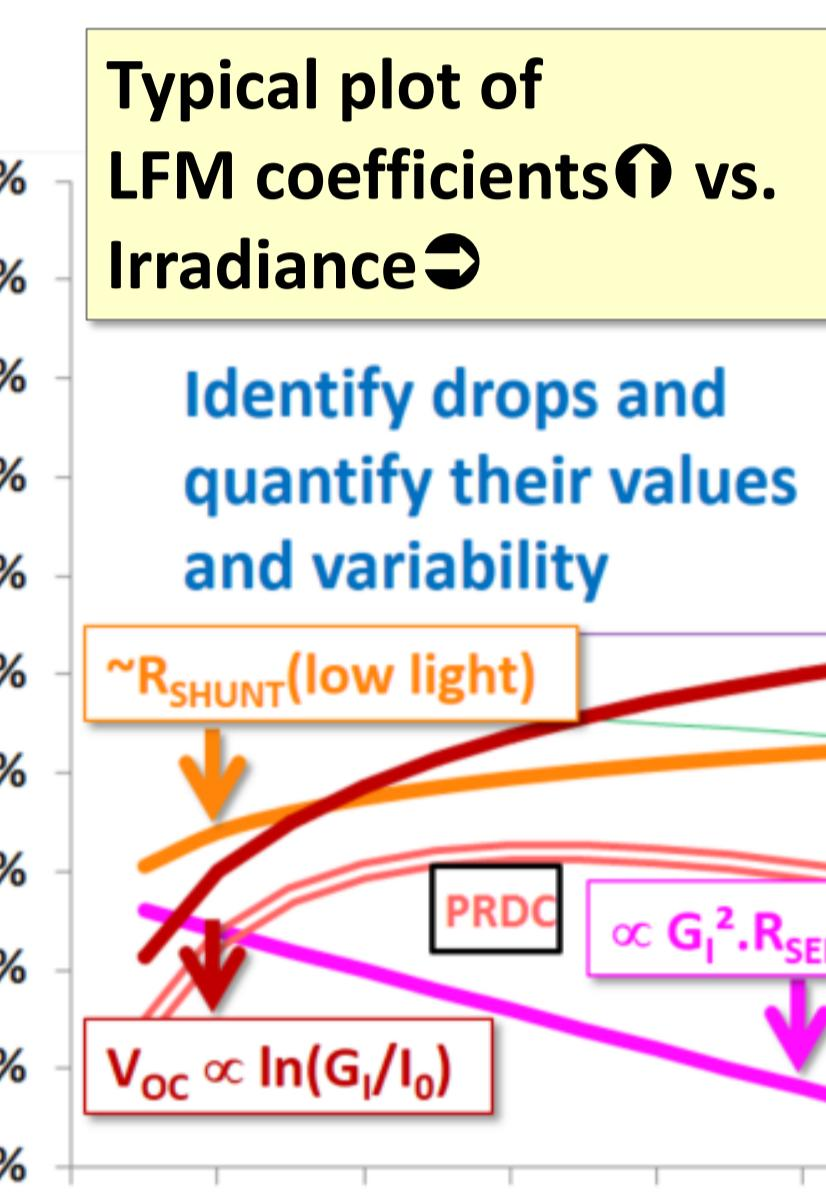
LFM values vs. irradiance show efficiency is affected by Low irradiance :  $nR_{SC}$  (dominated by  $R_{SHUNT}$ ) and  $nV_{OC,T}$
