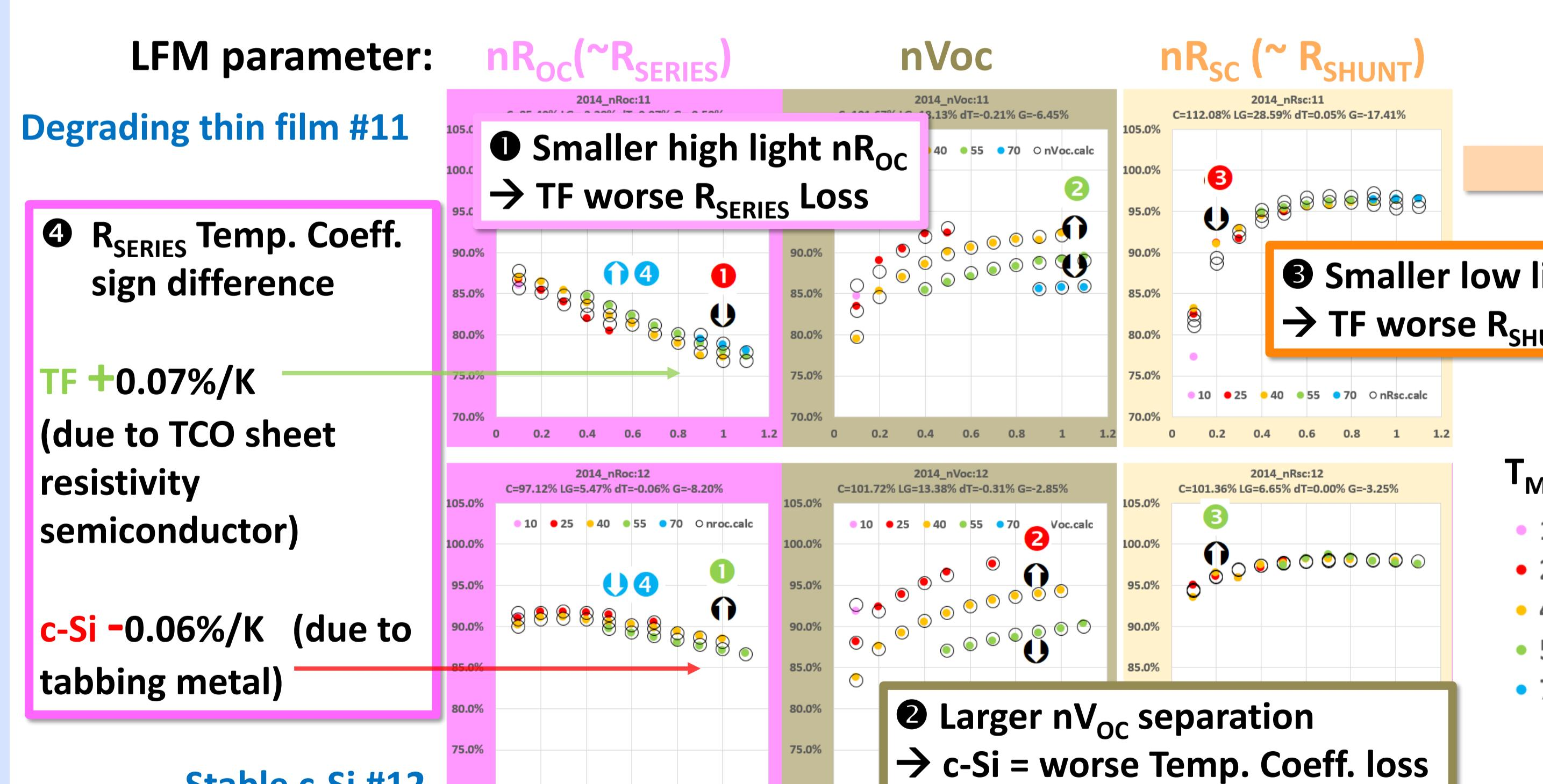
$nR_{SC}$  vs.  $Gi$  : Finding the cause and rate of drop of a degrading module 2013-16 (GI Measurements)
