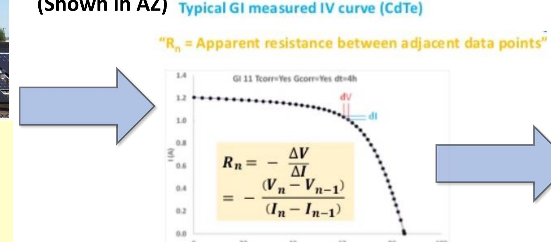
Checking IV data quality with Log Resistance-Voltage (RV) curves
