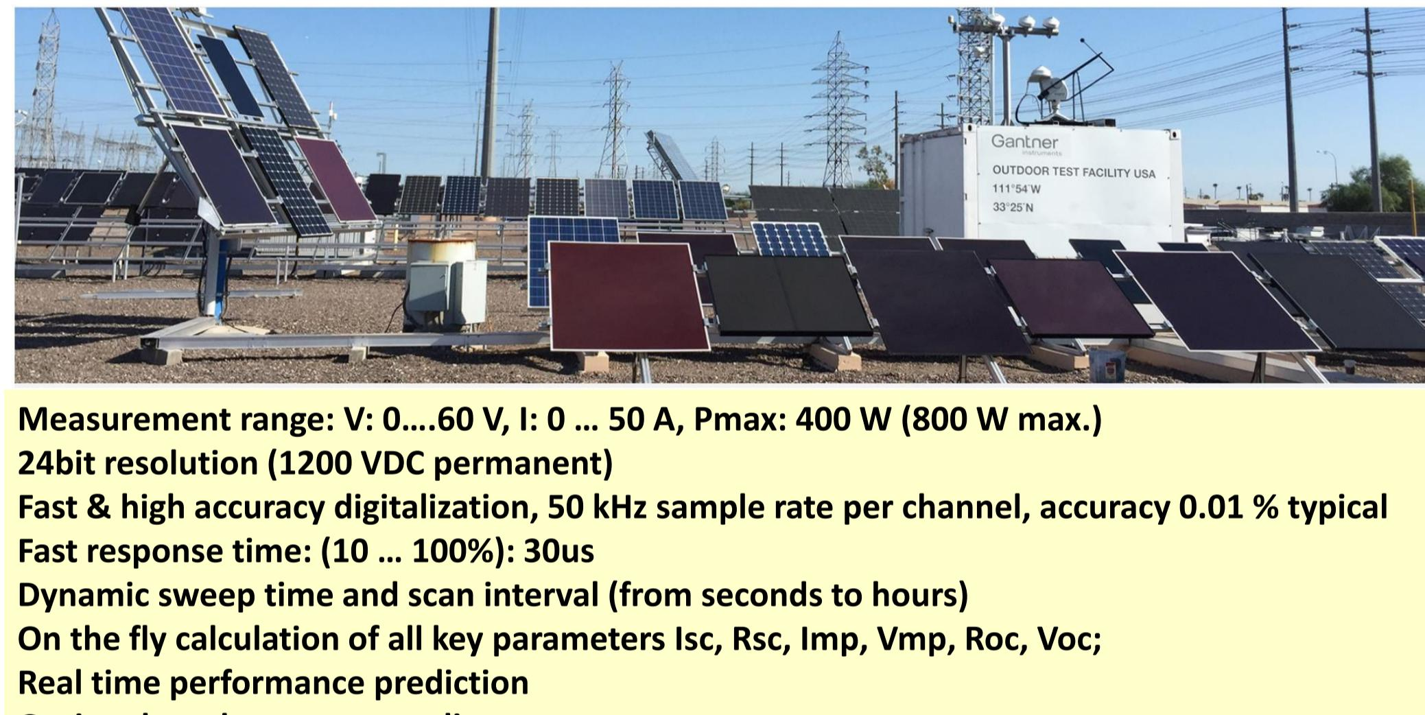
Smooth IV curves are needed for good  $R_{SC}$  and  $R_{OC}$  calculations
