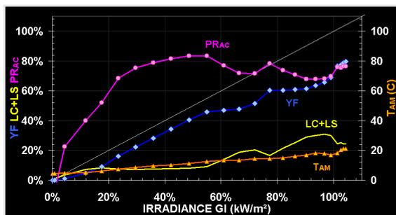
Fig 4. Rooftop 1.5kWp STC c-Si Array with 4kW Inverter on a Sunny morning in California versus Irradiance
