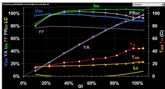
Fig 2. Derived Parameters from swept IV traces for a good c-Si module in Australia versus Irradiance.
