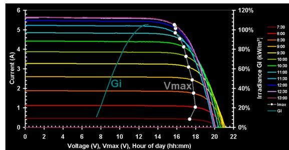
**Fig 1.** Swept IV traces every 30 minutes for a c-Si Module on a sunny morning in Australia showing the Irradiance versus time and the true  $V_{MAX}$  for every measurement.
