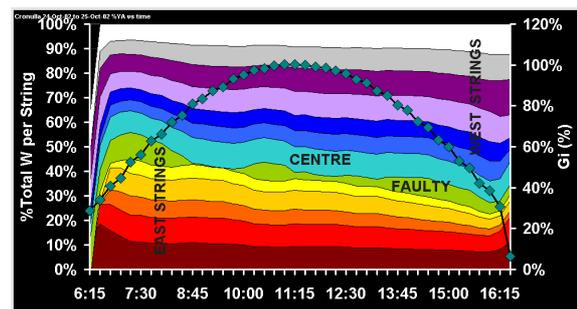
**Fig 7.** Variable Percentage of Total W from 13 strings and Horizontal Irradiance (as initially set up) on a curved roof, Winter in Australia
