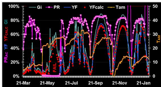
**Fig 6.** Good stability and performance from a c-Si Array in Tennessee except downtime 21<sup>st</sup> May.
