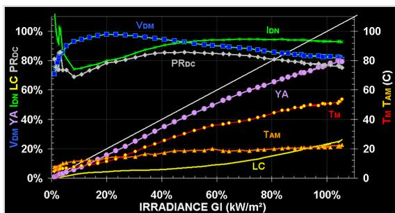
Fig 3. Derived Parameters from DC MPPT for a good c-Si module in Germany versus Irradiance.
