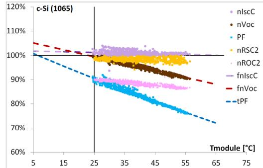
**Figure 2:** LFM-B coefficients and their gradients versus module temperature for a c-Si PV module at OTF1-CH.
