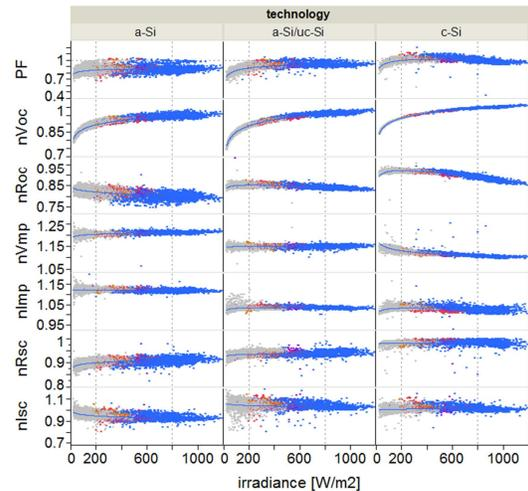
**Figure 3:** Performance factor (PF=mEff/rEff) and LFM parameters as a function of irradiance (Gi) for a-Si, a-Si/uc-Si and c-Si PV modules at OTF1-CH from 08/2009-08/2012.
