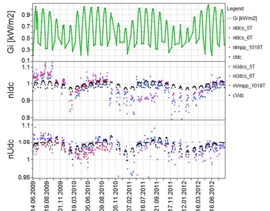
**Figures 7:** Stabilization of the a-Si arrays over 3 years with seasonal annealing of (a)  $n_{Idc}$  and a smaller change in (b)  $n_{Vdc}$  (hourly data).
