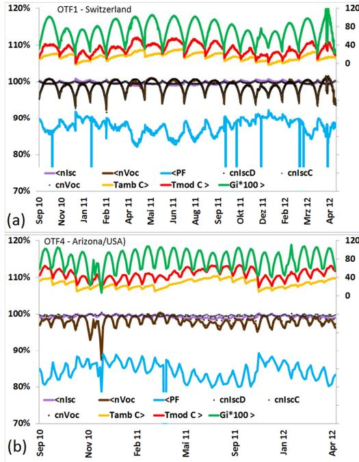
**Figure 6:** Irradiance ( $G_i$ ), ambient and module temperatures, PF, LFM-B parameters  $n_{Lsc}$ ,  $n_{Voc}$  and their fits over time for similar c-Si PV modules at OTF1-CH and OTF4-AZ (09/2010-04/2012).
