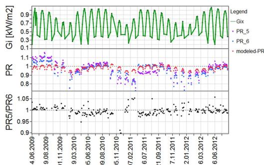
**Figure 8:** Comparison of Performance Ratio of plants 5 (pink) and 6 (blue) versus model (red) and ratio of PR5/PR6 (hourly data).
