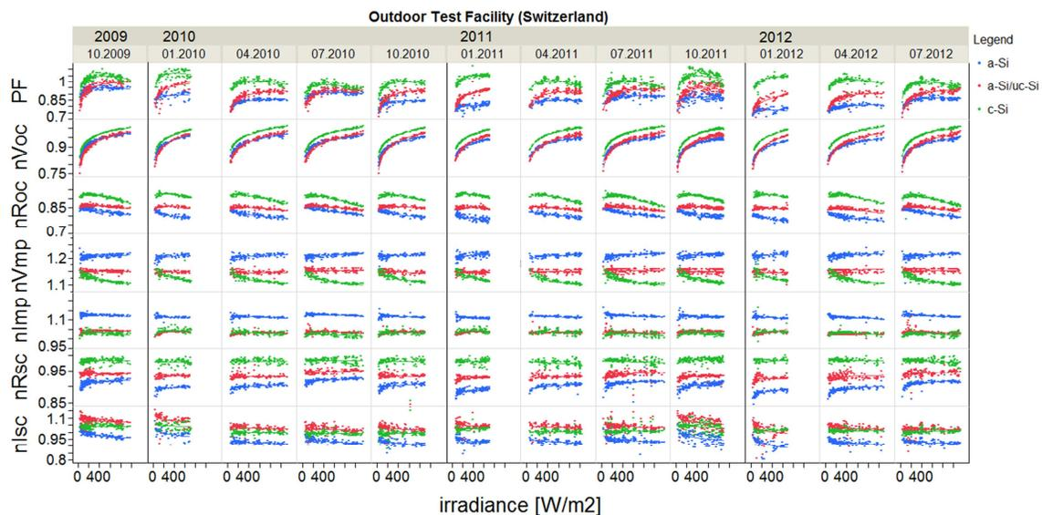
**Figure 4:** LFM-B parameters and PF versus irradiance for quarterly data from 10/2009 to 07/2012 for a-Si, a-Si/uc-Si and c-Si PV modules at OTF1-CH.
