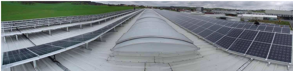
Figure 1: Panoramic view of the 83kWp AR vs Control test arrays in Germany
