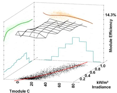
Figure 2: BP 7180 Efficiency vs module temperature and Irradiance.
