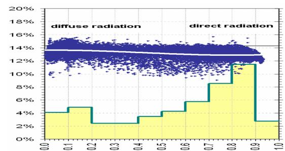
Figure 6) Module efficiency vs Beam Fraction (diffuse to the left, direct to the right)
