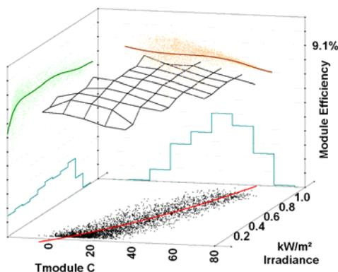
Figure 4: Competitor CIS Efficiency vs module temperature and Irradiance.
