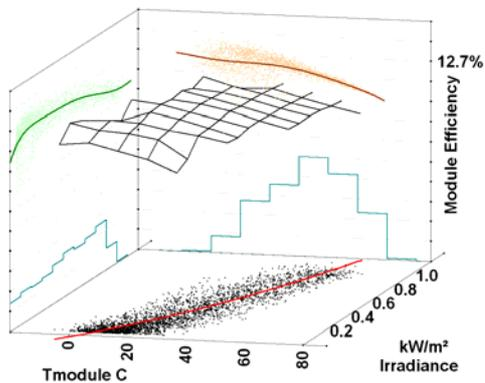
Figure 3: BP 3160 Efficiency vs module temperature and Irradiance.
