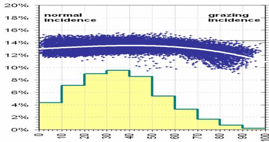
Figure 7) Module efficiency vs Angle of Incidence (°) Normal incidence to the left, grazing angle to the right
