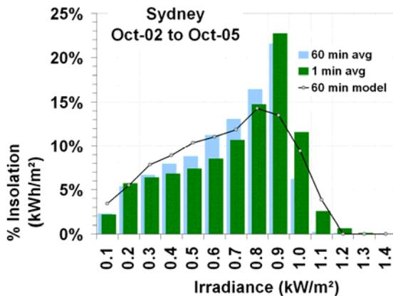
Figure 10: Distribution of irradiant energy  $\text{kWh/m}^2$  vs irradiance  $\text{kW/m}^2$  for a commercial hourly stochastic model (grey line) and measured hourly- (light blue histogram) and 1 minute-(dark green histogram) averaged data at Sydney, Australia. Measured data every minute 2002-2005
