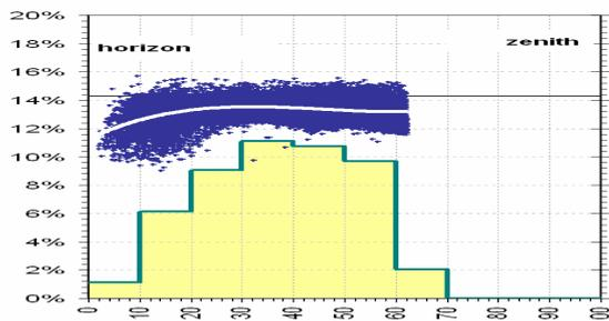
Figure 8) Module efficiency vs solar height (°) Low height to the left, zenith is 90°
