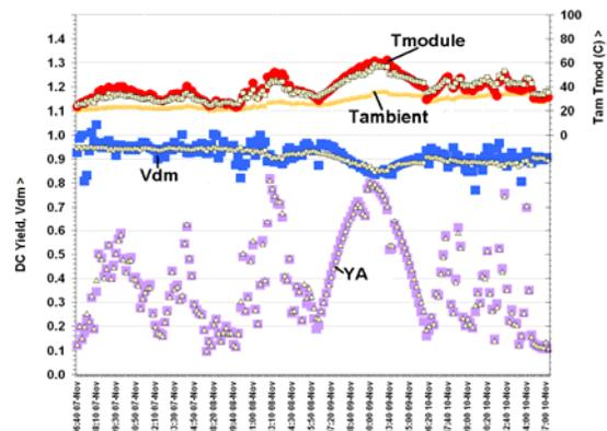
Figure 9: Measured and predicted performance of module versus time in Australia under varying weather conditions showing from top to bottom  $T_{module}$ ,  $T_{ambient}$ ,  $V_{dm}$ , YA.
