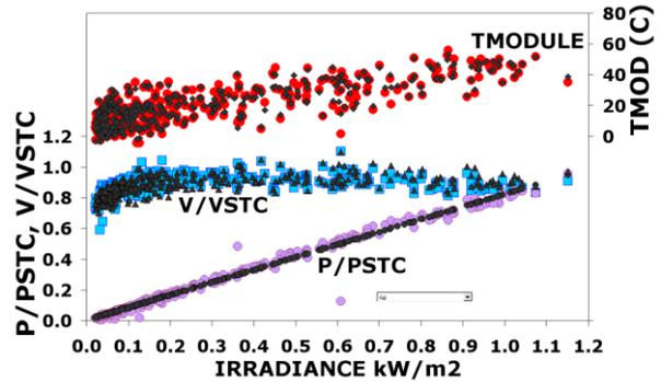
Figure 5: Empirical fits for temperature, voltage and dc yield for a mc-Si module at ISET
