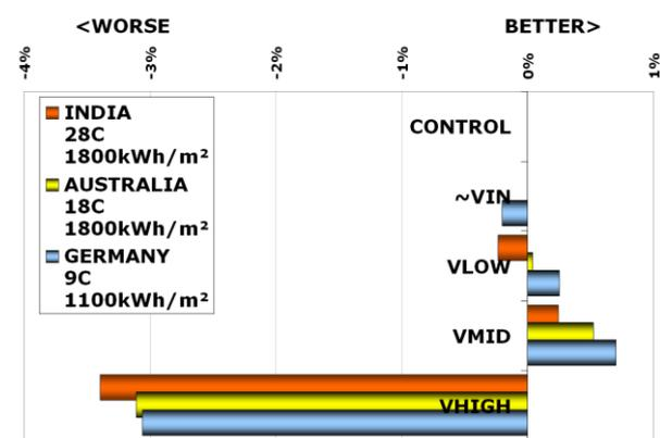
Figure 10: Energy yield changes at three sites from inverter efficiency modelling with input voltage,
