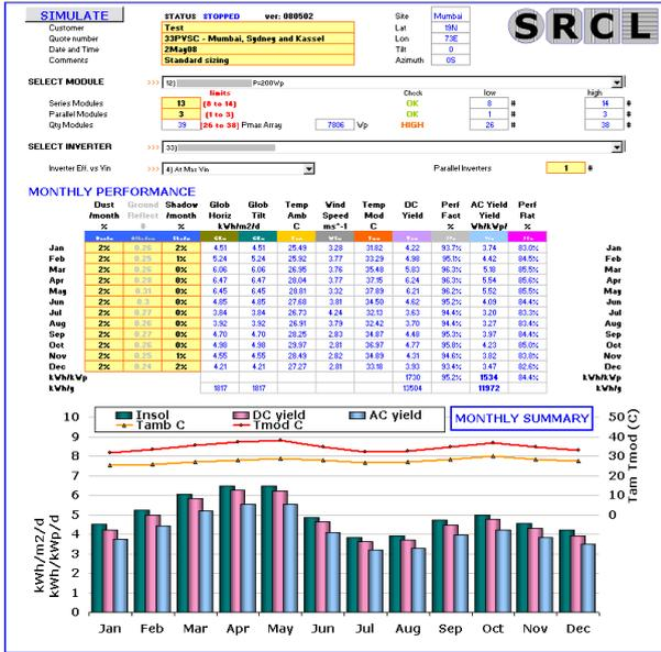
Figure 7: New sizing program to investigate inaccuracies and different modelling algorithms
