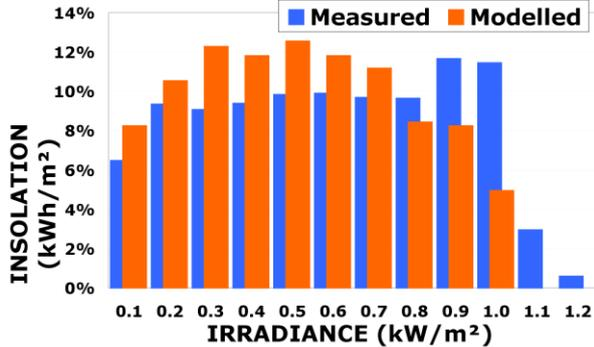
Figure 4: Measured (2004) vs a meteorological database modelled percentage tilted plane insolation vs irradiance in central Germany.
