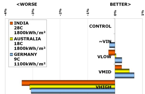
Figure 10: Energy yield changes at three sites from inverter efficiency modelling with input voltage,
