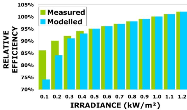
Figure 3: Measured vs a sizing program model for relative efficiency vs irradiance for mono Si module
