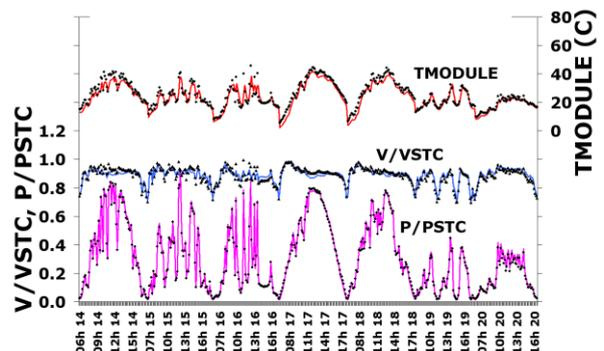
Figure 6: Measured and predicted  $T_{MODULE}$ ,  $V_{DM}$  and  $YA$  for mc-Si module for 7 days in September 2004 at ISET.
