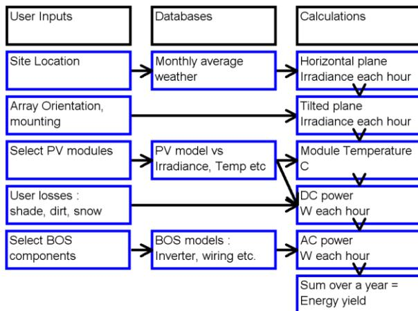
Figure 1: Simplified flow chart showing user input, database and calculation stages used by many sizing programs to predict energy yields.
