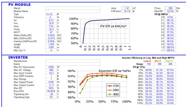
Figure 8: Input screens for PV and inverters.
