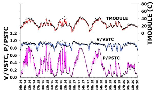
Figure 6: Measured and predicted  $T_{\text{MODULE}}$ ,  $V_{\text{DM}}$  and  $YA$  for mc-Si module for 7 days in September 2004 at ISET.
