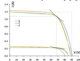
Figure 1: PVSP predicted thin film IV curves @ 1000 and 200W/m<sup>2</sup>
