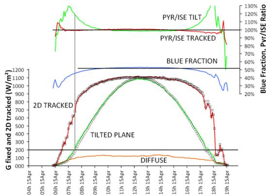
Figure 13: Irradiance from a pyranometer vs. corrected @AM1.5 ISE sensor, tilted plane vs. 2D tracked for a good irradiance day in April at Oerlikon Solar's OTF4-AZ
