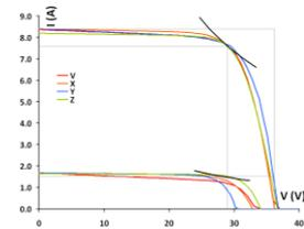
Figure 2: PVSP predicted c-Si IV curves @ 1000 and 200W/m<sup>2</sup>
