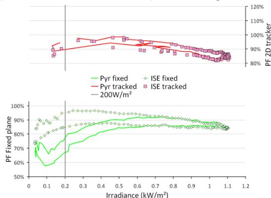
Figure 14: Apparent change in low light behaviour due to sensor choice for a c-Si at Oerlikon Solar's OTF4\_AZ
