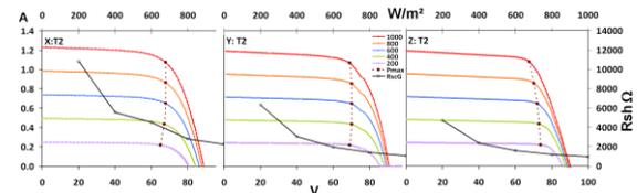
Figure 3: IV curves (colours - lower and left axes) of a thin film module with  $R_{SC}$  vs. irradiance (black - right and upper axes) from 3 PVSPs X, Y and Z
