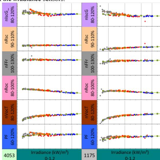
Figure 8: LFM fits to an a-Si:uc-Si module vs. Irradiance at OTF4-AZ (left 4053) and OTF1-CH (right 1175).
