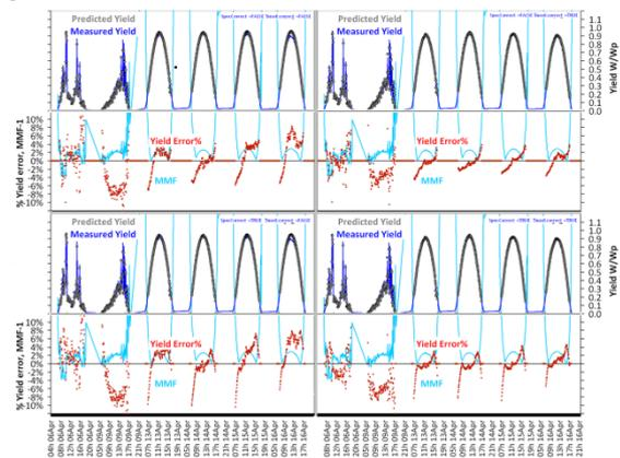
Figure 10: Energy yield LFM fits to an a-Si:uc-Si module at OTF4-AZ – temperature correction (left=no, right=yes); spectral correction (upper=no, lower = yes)
