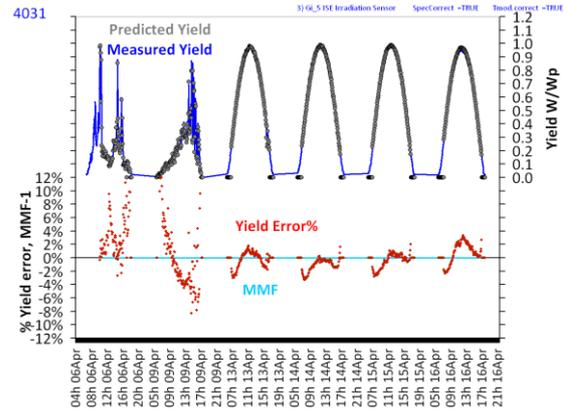
Figure 9: Energy yield LFM fits to a c-Si module at OTF4-AZ right
