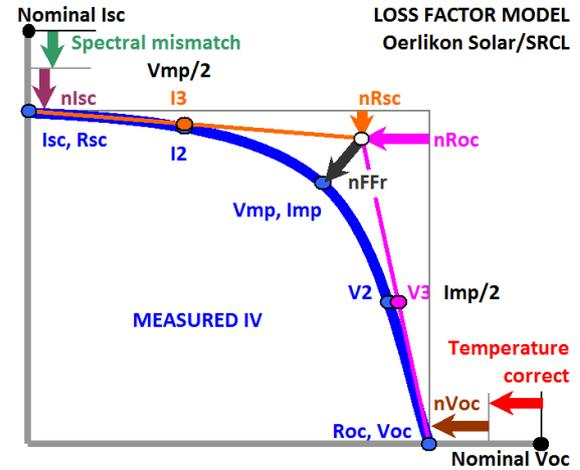
Figure 6: Identifying the 7 independent normalised coefficients that determine the performance factor in the LFM.
