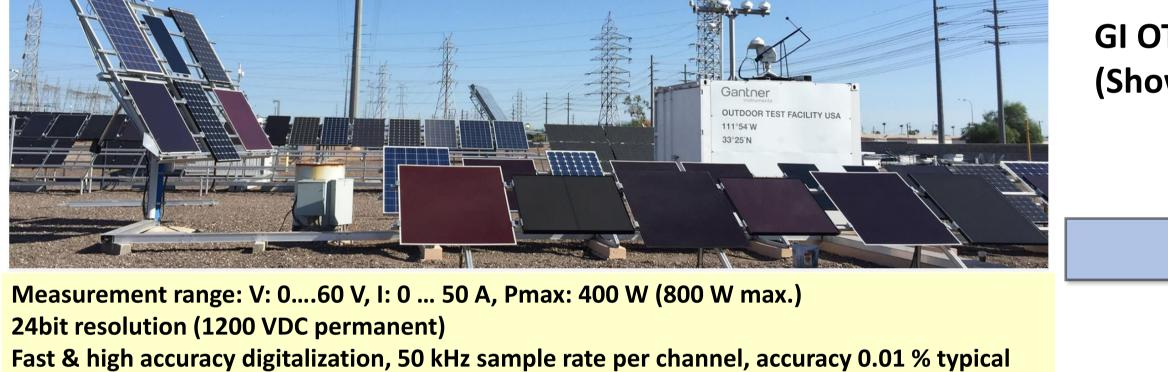
Smooth IV curves are needed for good R<sub>sc</sub> and R<sub>oc</sub> calculations Checking IV data quality with Log Resistance-Voltage (RV) curves GI data much smoother than NREL's Daystar and therefore easier to fit.
