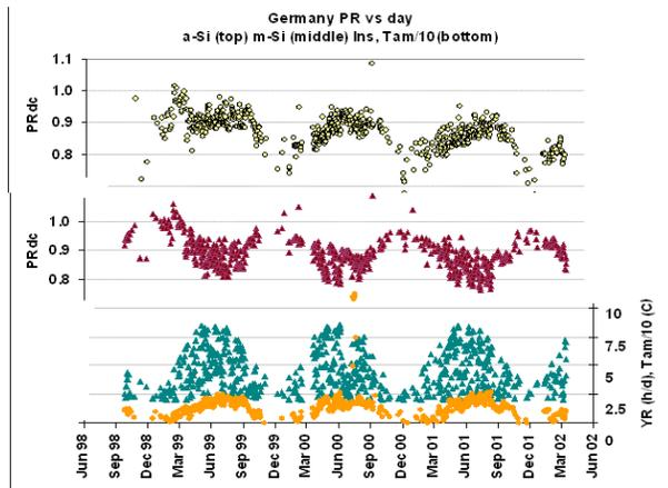
Figure 2: Daily Performance Ratio of a single junction a-Si module and a multi-crystalline silicon module for three years in Germany.
