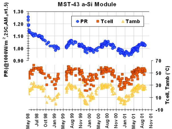
Fig. 1. Performance Ratio (PR) for a tandem junction amorphous silicon module against time and temperature.
