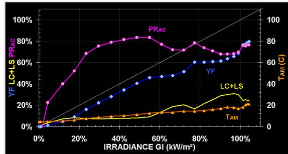
**Fig 4.** Rooftop 1.5kWp STC c-Si Array with 4kW Inverter on a Sunny morning in California versus Irradiance
