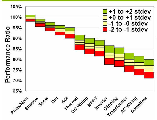
Estimate 3sigma distribution from previous graph for loss in a PV System
