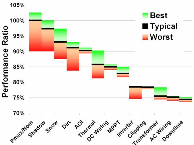
High and low limits for loss in a typical PV System
