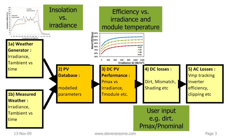
How simulation programs usually calculate kWh/kWp (Matrix method)
