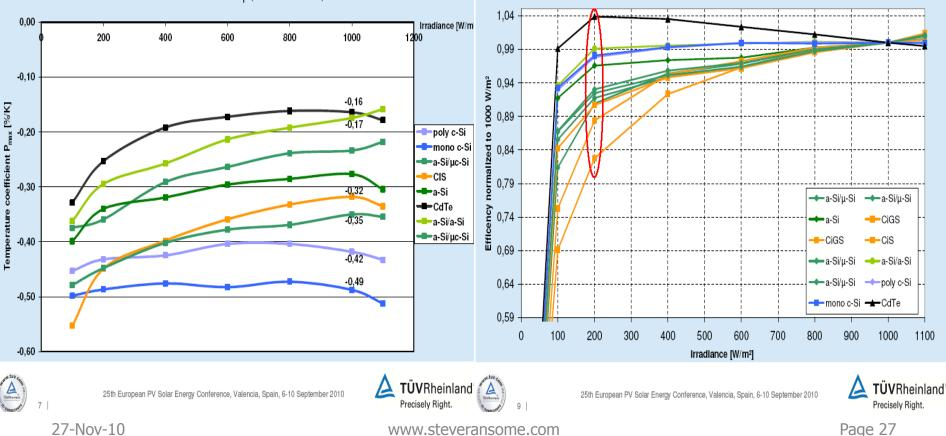
Indoor Measurements for Different  $G_{I}$  (IEC 61853)
