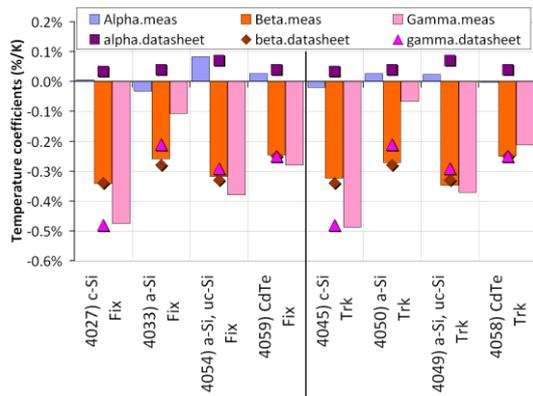
**Figure 5b:** Measured outdoor temperature coefficients vs. nominal datasheet values for different PV modules under real weather conditions at OTF4-AZ – left are fixed plane, right are 2D tracked equivalents.
