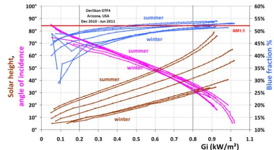
**Figure 2:** Blue fraction, AOI and Solar height vs. irradiance each month for clear sky days at OTF4-AZ.
