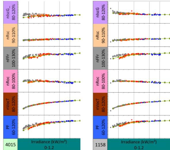
**Figure 8:** LFM fits to a CIGS module vs. Irradiance at OTF4-AZ (left 4015) and OTF1-CH (right 1158).
