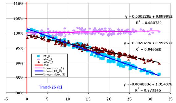
**Figure 4a:** Outdoor temperature performance of  $nI_{SC,G}$ ,  $nV_{OC}$  and PF vs. temperature ( $T_{MODULE}-25^\circ C$ ) for c-Si.
