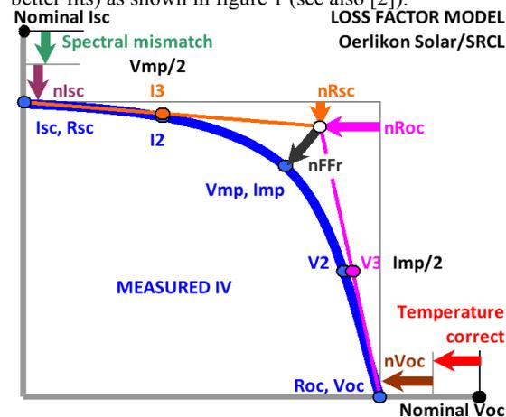
**Figure 1:** Determining the normalised independent loss factors ( $n_{I_{SC}}$ ,  $n_{R_{SC}}$ ,  $n_{FFR}$ ,  $n_{R_{OC}}$  and  $n_{V_{OC}}$ ) with two corrections (spectral mismatch and temperature) from a measured IV curve.
