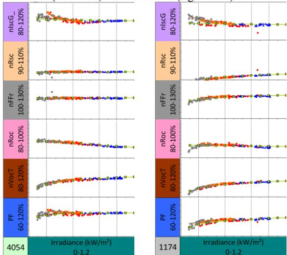
**Figure 9:** LFM fits to an a-Si/uc-Si module vs. Irradiance at OTF4-AZ (left 4054) and OTF1-CH (right 1174).
