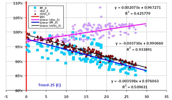
**Figure 4b:** Outdoor temperature performance of  $nI_{SC,G}$ ,  $nV_{OC}$  and PF vs. temperature ( $T_{MODULE}-25^\circ C$ ) for a Thin Film.
