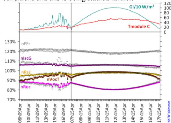
**Figure 12:** Fitted (colour) vs. measured (black) loss factor parameters and weather data for a thin film module measured at OTF4-AZ showing good agreement for a diffuse and a clear day in April
