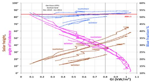
**Figure 3:** Blue fraction, AOI and Solar height vs. irradiance each month for clear sky days at OTF1-CH.
