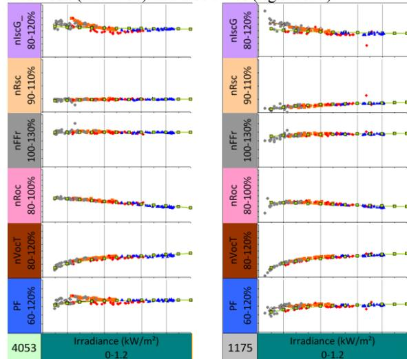
**Figure 10:** LFM fits to an a-Si/uc-Si module vs. Irradiance at OTF4-AZ (left 4053) and OTF1-CH (right 1175).
