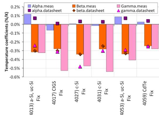
**Figure 5a:** Measured outdoor temperature coefficients vs. nominal datasheet values for six different PV modules under real weather conditions at OTF4-AZ.
