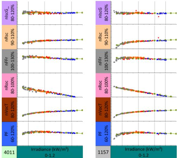
**Figure 7:** LFM fits to a CdTe module vs. Irradiance at OTF4-AZ (left 4011) and OTF1-CH (right 1157).
