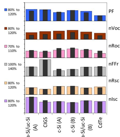
**Figure 11:** Five fitted loss factor coefficients for various modules at OTF4-AZ
