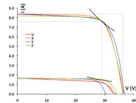
Figure 2: PVSP predicted c-Si IV curves @ 1000 and 200W/m<sup>2</sup>
