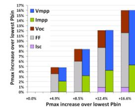
Figure 5: CdTe bin values from manufacturer's datasheet
